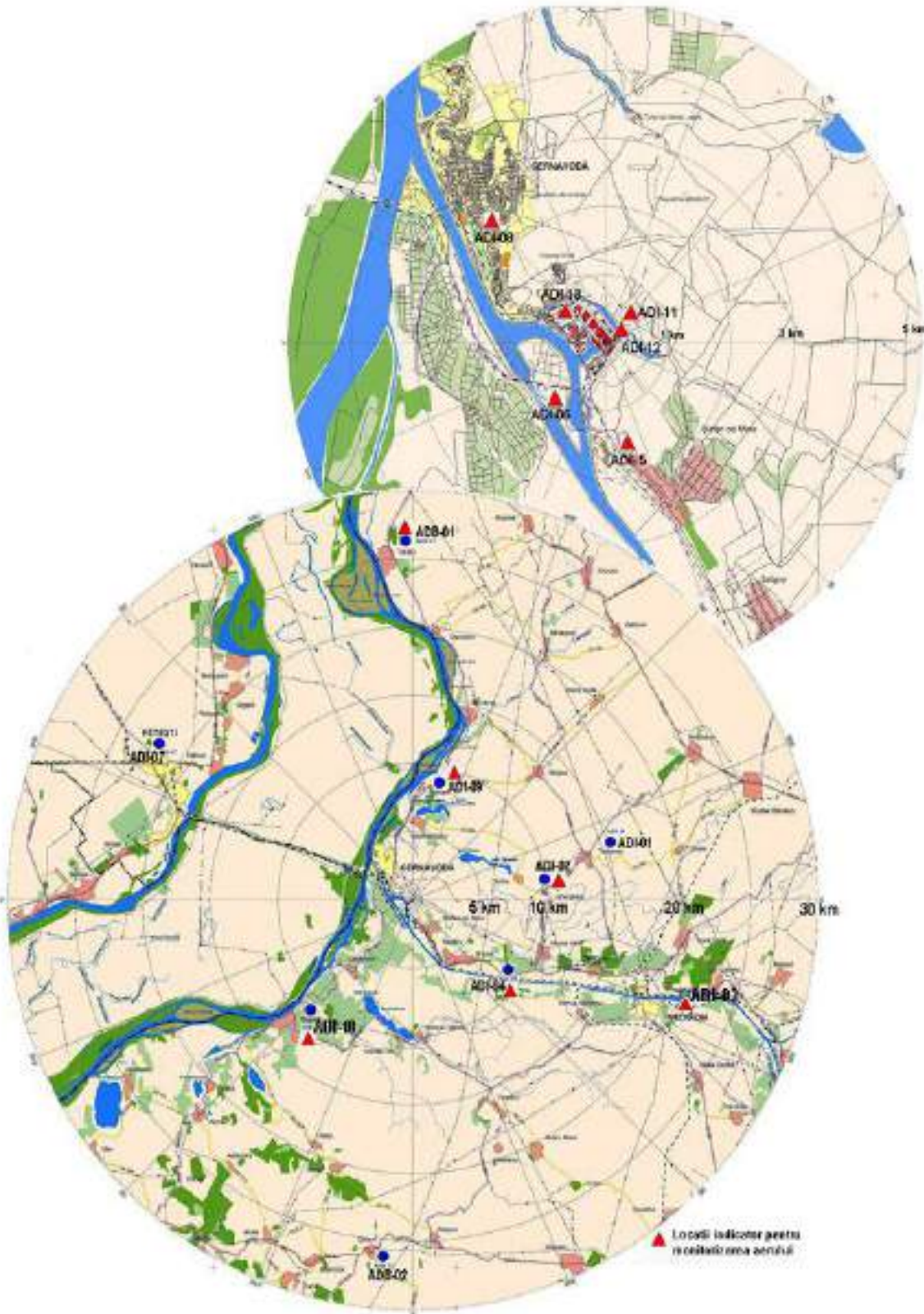
Figure 1.4.14.2 Location of investigation points for tritium concentrations in the air according to the environmental radiological monitoring program by Cernavoda NPP
