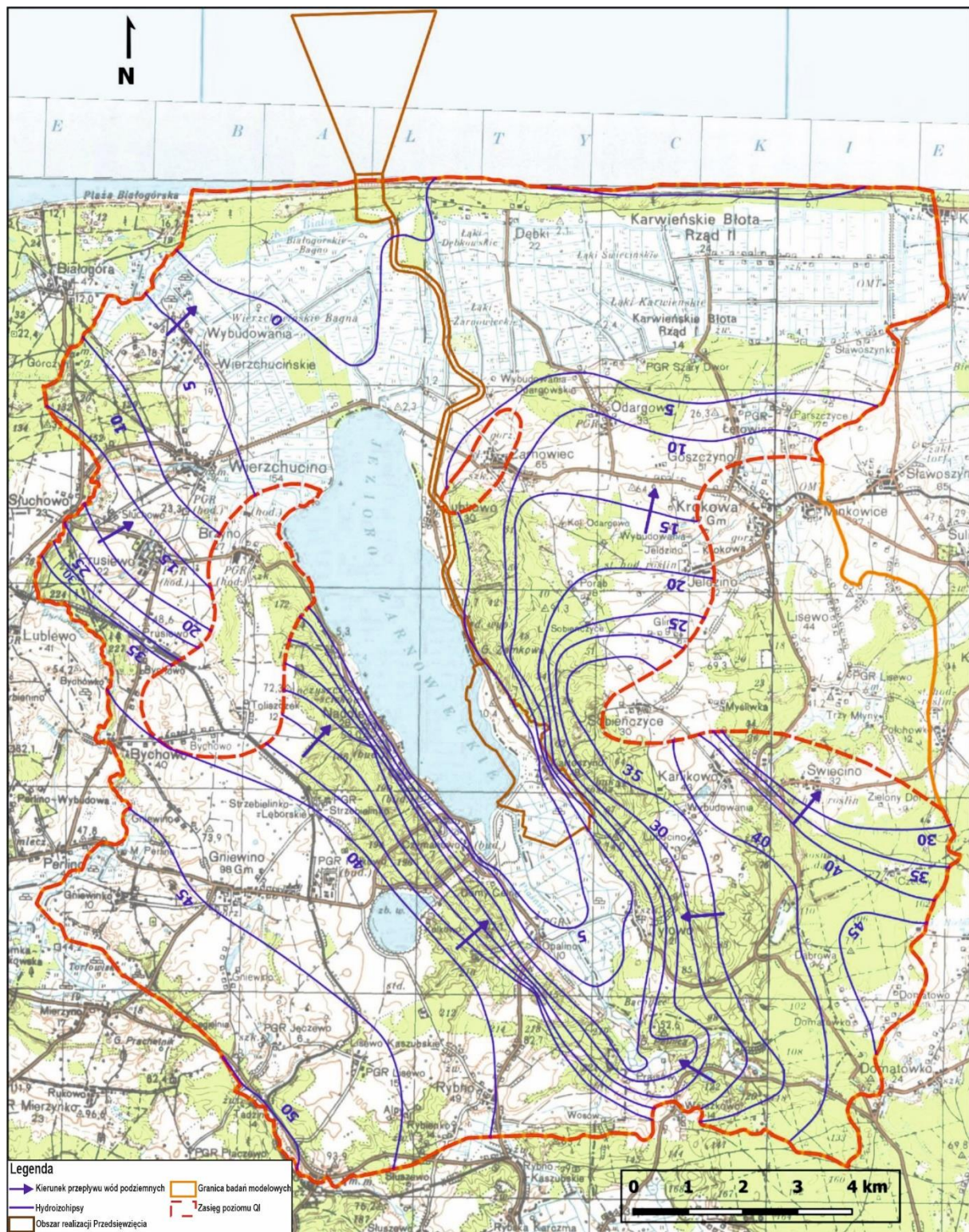
Figure VI.3.3.5- 2 Map of the hydroisohypses of the first Q1 aquifer Source: In-house study
