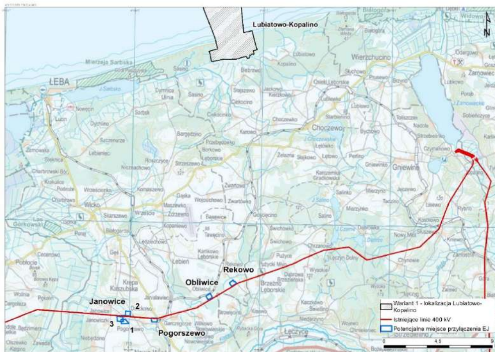
Figure II.12.3-4 Potential variants for the location of the 400 kV electrical substation forming a connection point between the NPP and the National Power System. Variant 1 – Lubiatowo – Kopalino site [Legend: Grey – Variant 1 Lubiatowo-Kopalino site, Red line – existing 400kV line, Blue – Potential locations for NPP connection]
