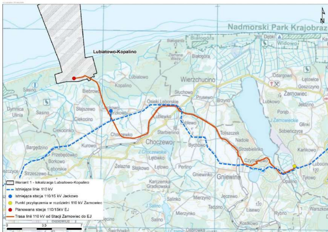
Fig. II.12.3- 1 Proposed routing of the 110 kV cable line along the section from the 400 kV Żarnowiec electrical substation to the Project execution area. Variant 1 – Lubiatowo – Kopalino site [Legend: Grey – Variant 1 Lubiatowo-Kopalino site, Blue line – existing 110kV line, Red line – 100kV route from Żarnowiec substation to NPP, Blue dot – Existing Jackowo 110/15kV substation, Yellow dot – Connection point at 100kV Żarnowiec substation]
