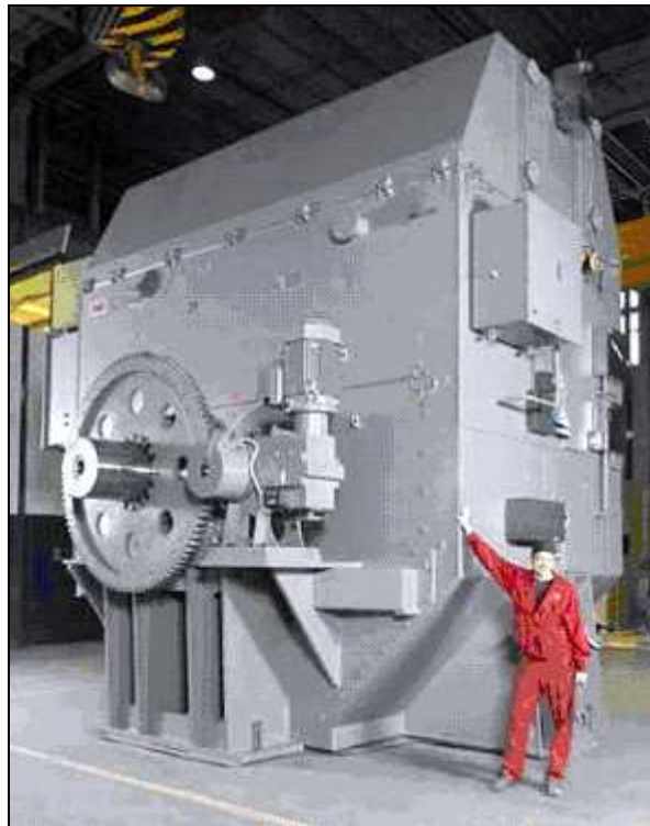
Figure 3.26: A compressor motor with a rated output of 24 MW [95, Savolainen, 2005]
