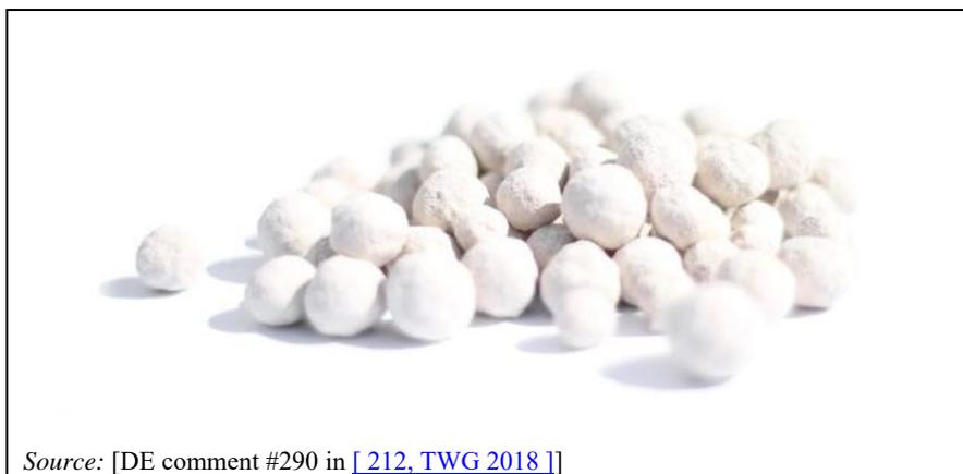
**Figure 17.21: Pelletised natural molecular sieve (zeolite)**
