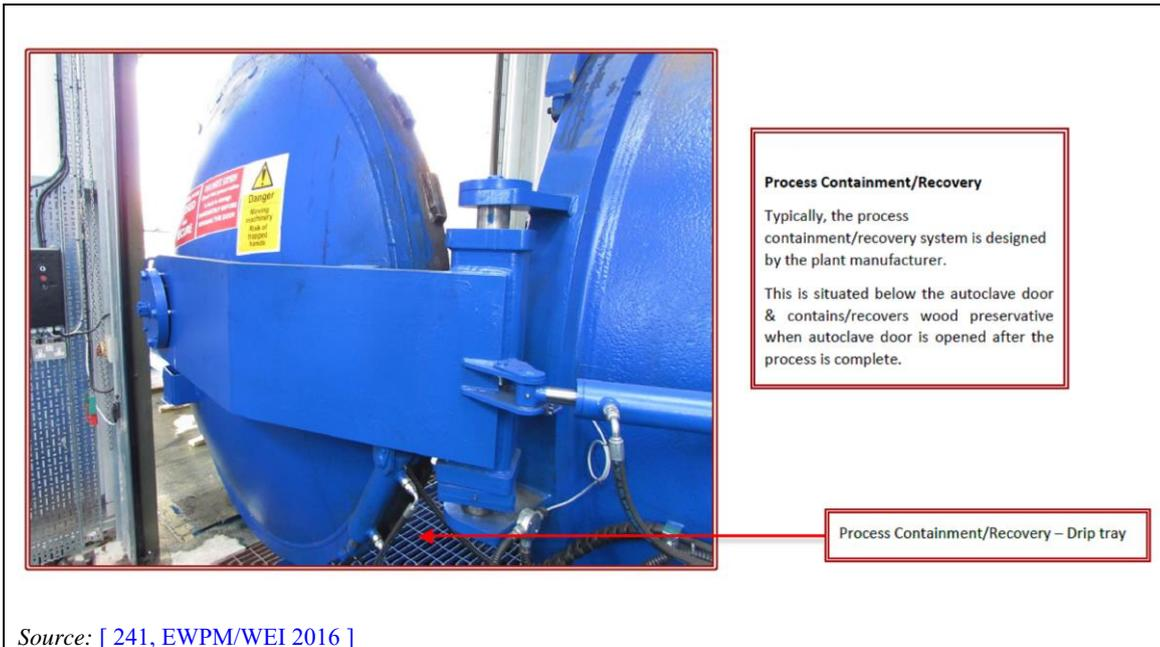
**Figure 15.23:** Example of a drip tray underneath an autoclave door
