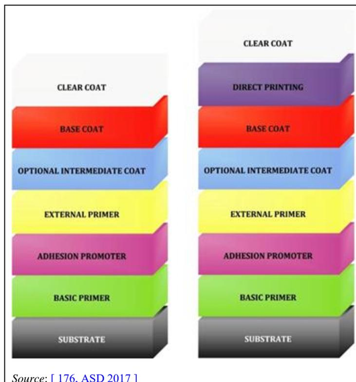
**Figure 5.11: Comparison of BCCC (base coat / clear coat) system with direct printing in the BCCC system**
