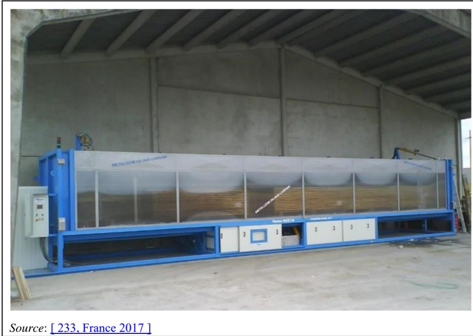
**Figure 15.7: Wood in closed spraying tunnel**
