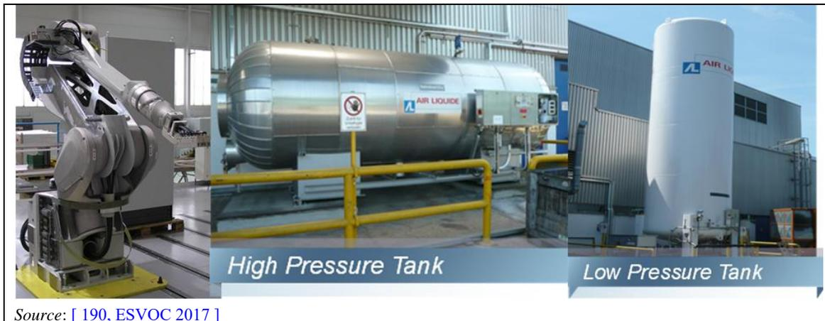
Figure 17.14: (a) Applicator robot, (b) High-pressure CO<sub>2</sub> tank, (c) Low-pressure CO<sub>2</sub> tank
