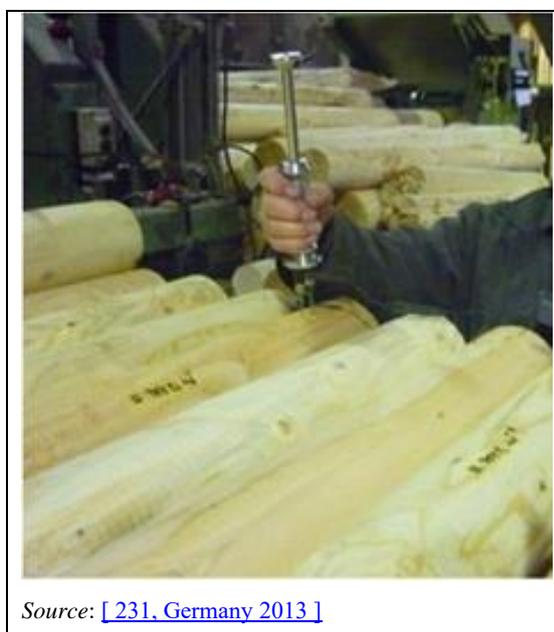
**Figure 15.27:** Manual wood moisture measurement
