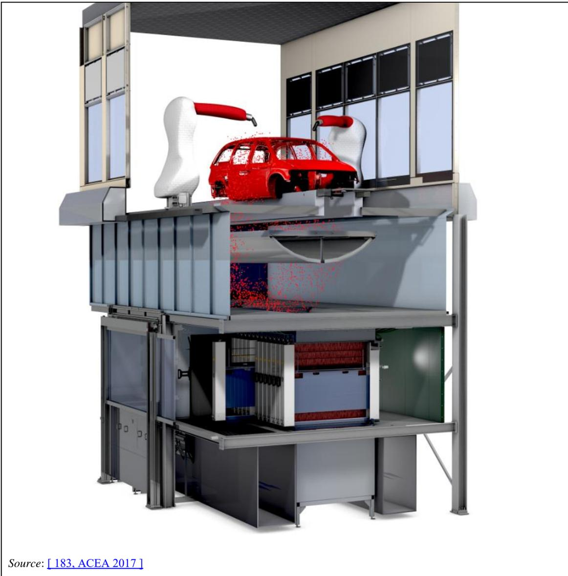
**Figure 2.45: Rinsed electrofilter system**
