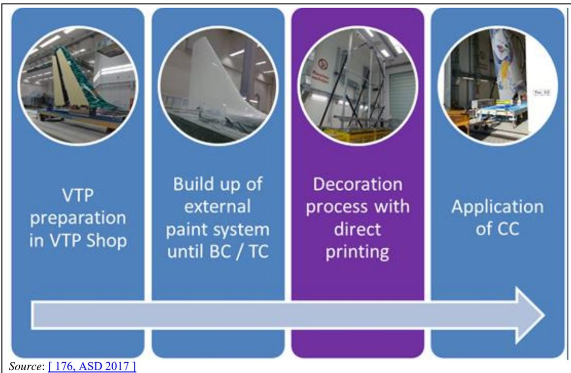
Figure 5.10: Process chain including direct printing
