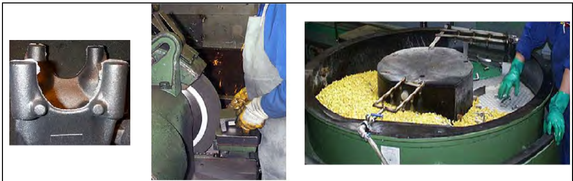
Figure 2.51: Burrs (l.) and their removal using a grinding stone (m.) and slide grinding (r.) [237, HUT, 2003]
