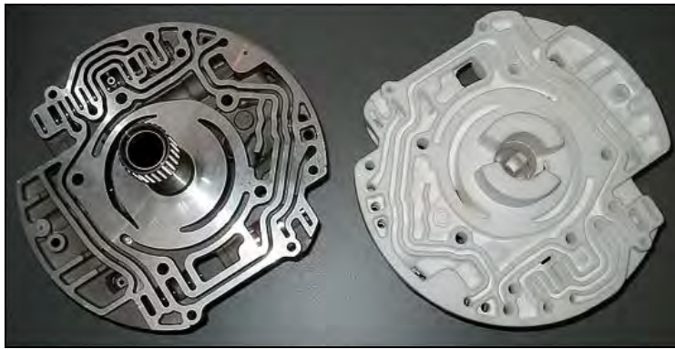
Figure 2.37: Expendable polystyrene pattern (r.) for the Lost Foam process and an example of a casting produced by the Lost Foam method (l.) [237, HUT, 2003]
