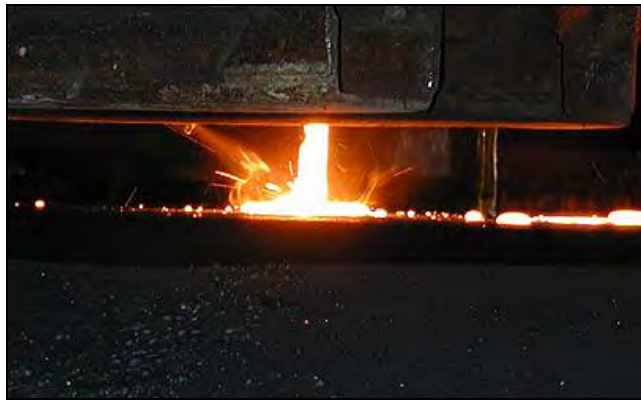
Figure 2.24: Inoculation during pouring [237, HUT, 2003]
