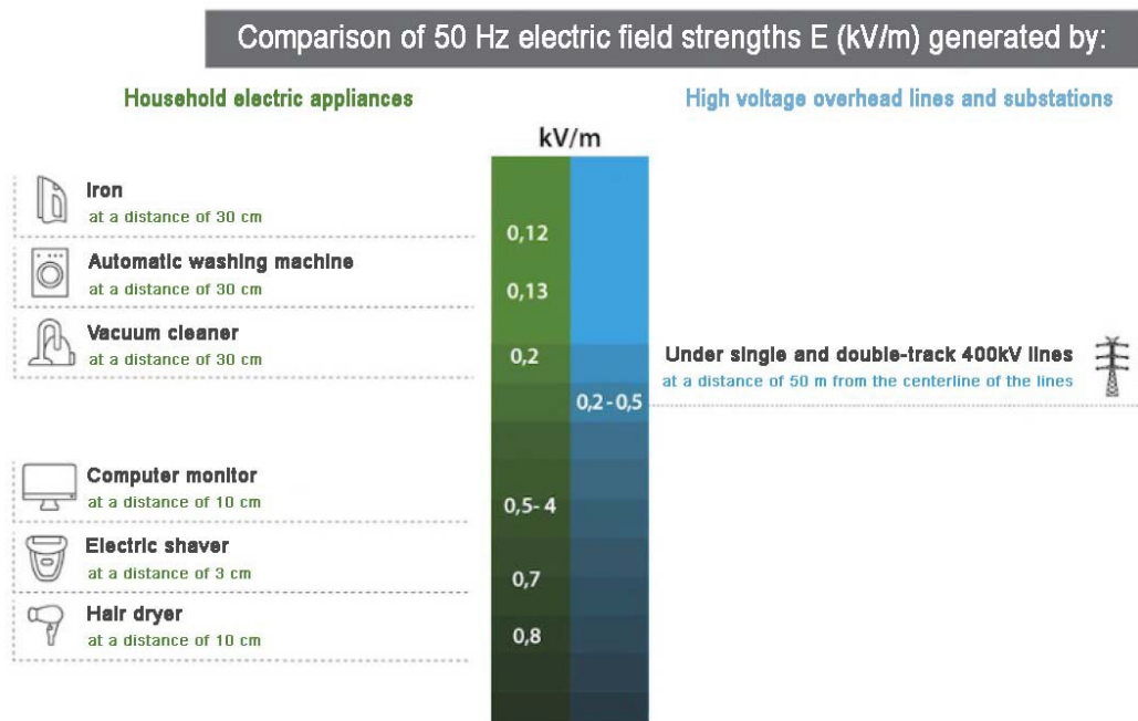
Figure 28. Comparison of 50 Hz electric field strengths (kV/m) generated by household electric appliances and extra high voltage overhead lines (Source: http://budowalini400kv.pl/ ).
