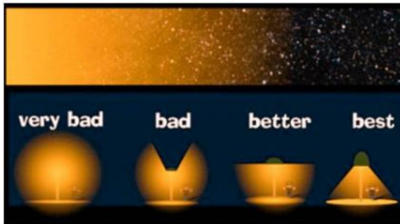
Figure no.7-1 Example of a lighting system suitable for concentrating the dispersion exclusively on the roadway
