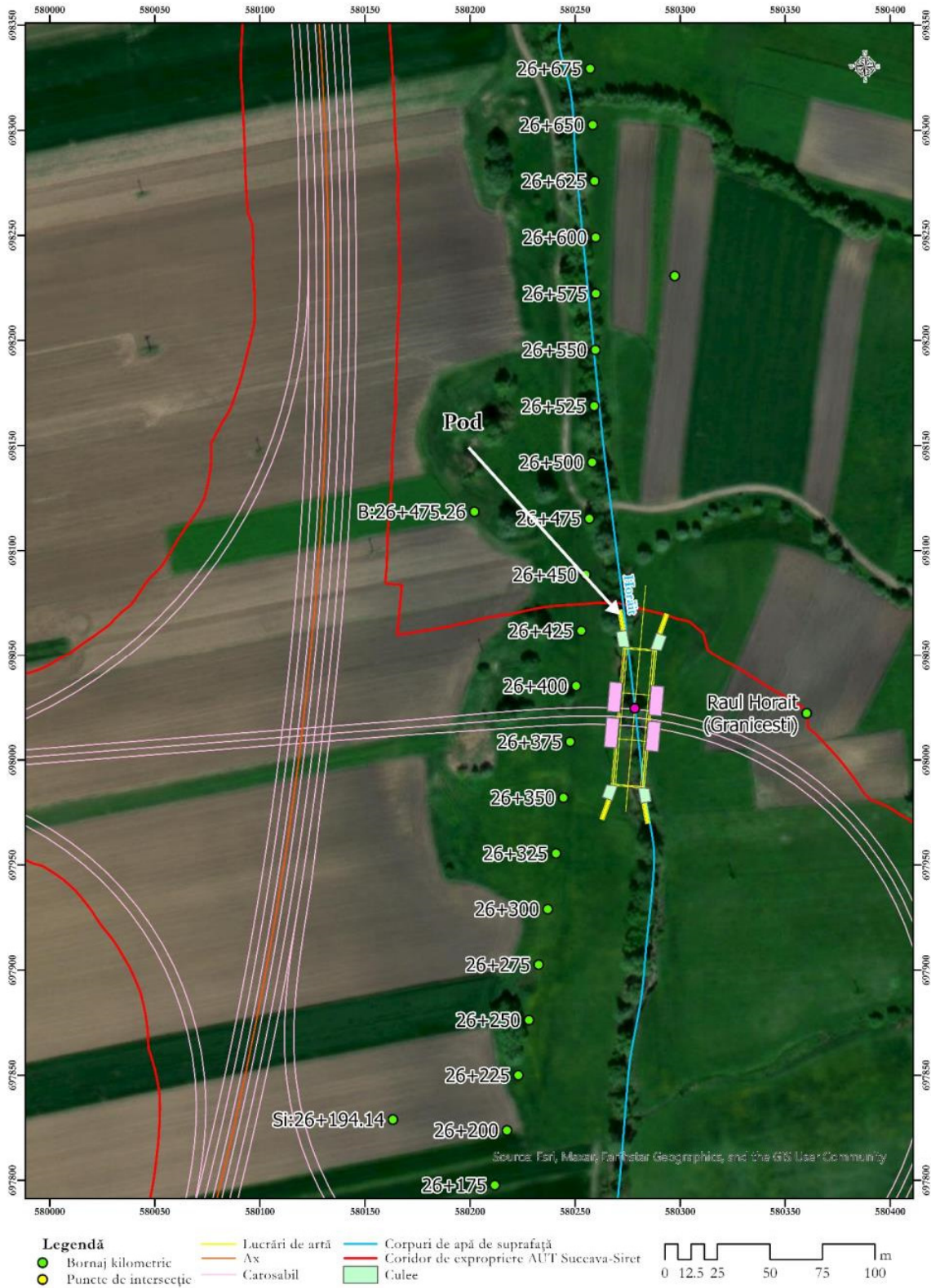
Figure no.2-8 Bridge designed on the Horaiț water body – RORW12-1-17-24A_B1 (km 35+950 – km 36+090)
