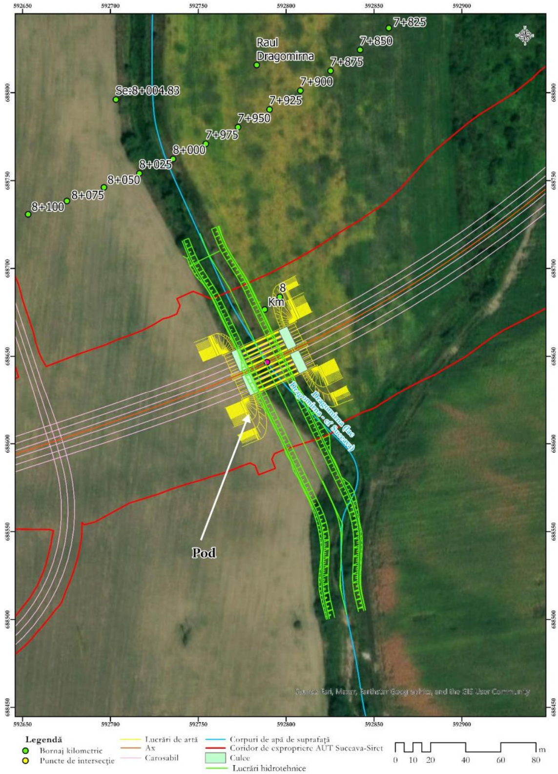
Figure no.2-3 Bridge designed on the Dragomirna water body (Lake Dragomirna – cf Suceava) – RORW12-1-17-30_B3
